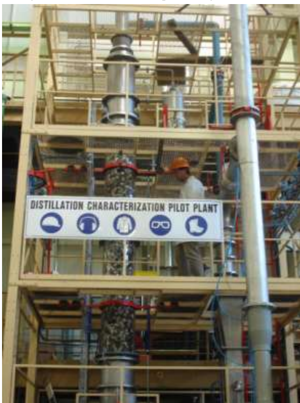
One of the distillation columns in the Department that facilitates cutting-edge research in separation technology in the chemical industry.
