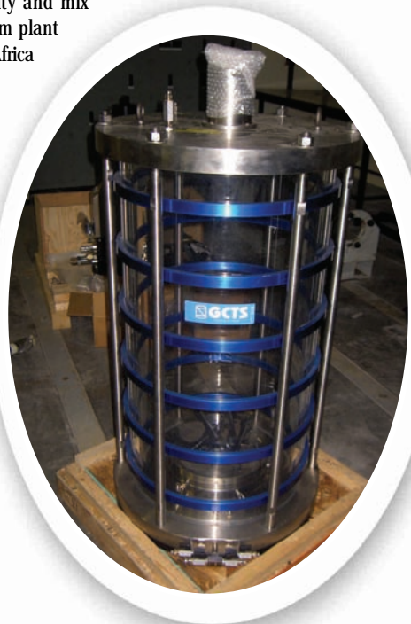
Large Triaxial for granular material specimens 300 mm diameter and 600 mm high.
