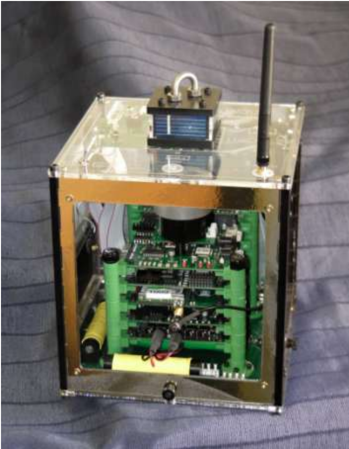
Edu_Satellite is an educational satellite that is used by the Department of Electrical and Electronic Engineering in the postgraduate Satellite Systems coursework.
